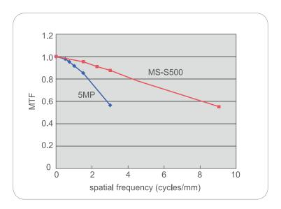
Fig. 5 Measured MTFs of horizontal direction (the sub-pixel chain direction) on MS-S500 and a conventional 5MP LCD
