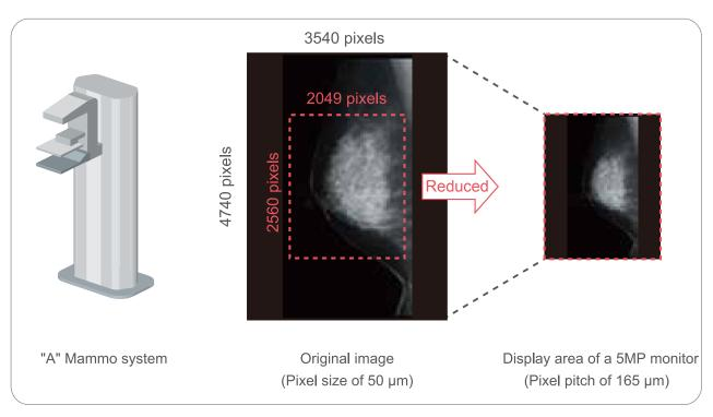
Fig.1 Depiction image when an original image consists of more pixels than a monitor in full-screen. It is reduced to only 31% of the original.
