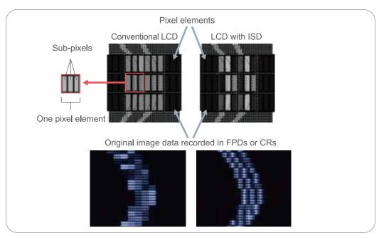
Fig.2 Mechanism of ISD and comparison of the images of three fine lines
