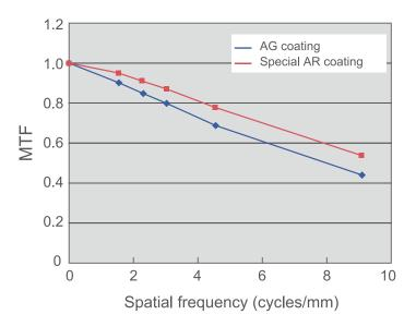
Fig.5 Focus characteristics measured by 5MP monitor
