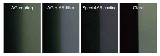
Photos of the LCD surfaces reflecting a piece of white paper
