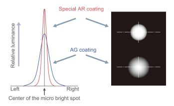
Fig.2 Illustration of the displayed micro bright points
